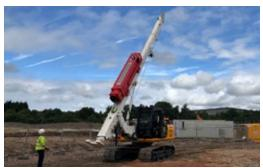
Introducing the all new BSP JX25 piling rig based on a 20 tonne excavator. Designed for driving most types of foundation piles.
